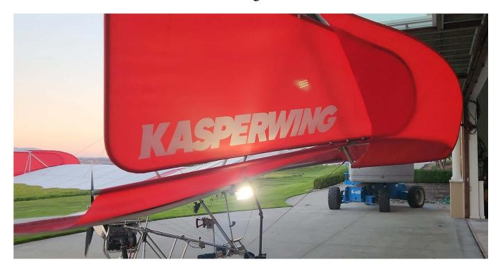
These are inexpensive, battery-operated strobes mounted to brackets on each wing tip. The strobes have several blinking modes and a mode for color (white, red, green). The batteries are recharged using a USB cable and last about 4 hours before recharging is needed. The strobes make it a lot easier to be seen by other aircraft even in daylight.
