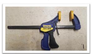
consists of several in the 6", 12" and 18" sizes, including one with a reversing head that acts as a spreader bar.
