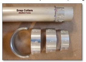
Rather than drilling through and through, I sometimes find it faster and more accurate to mark and then drill holes from both sides.
